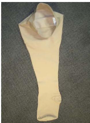
FIGURE 4 Circular knit knee high garment Shaped by forming the heel and varying inlay yarn tension and stitch height during knitting.
